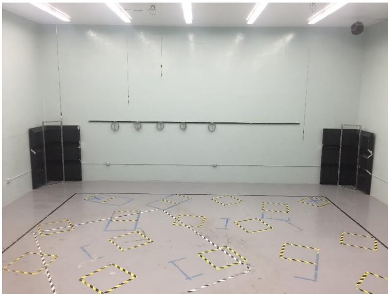
ABM CornerSorber Low-Frequency Absorption test, NWAA Labs, 8 September, 2016
